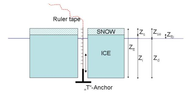
Figure 1: Definition of different variables related to sea-ice thickness  $(z_i)$ , including total thickness  $(z_{tt})$ , snow depth  $(z_s)$ , surface elevation  $(z_{se})$ , and freeboard  $(z_{fb})$ . Also shown is direct measurement of these variables in a single drill hole (Figure from Haas and Druckenmiller, 2009).
