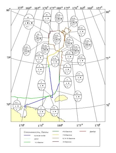
Figure 3: Example of an ice map, prepared from visual observations during an icebreaker's winter expedition north of Wrangell Island.
