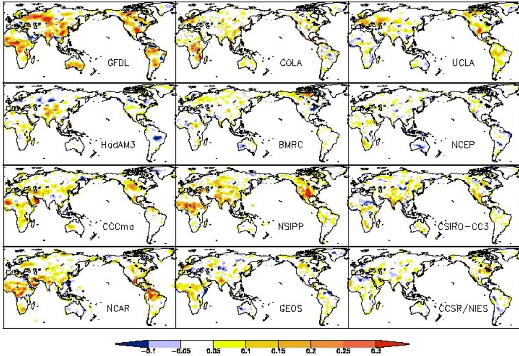
**Figure 1.** The " $\Omega(S) - \Omega(W)$ " diagnostic from GLACE-1, showing the degree to which precipitation variations respond to soil moisture variations. (From Koster et al., 2006.)
