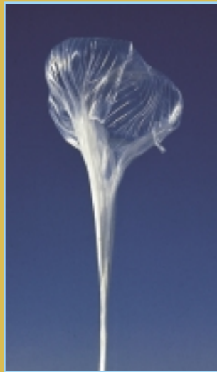
Super-pressure balloons carry instruments up to the stratosphere to measure temperature and water vapour.
