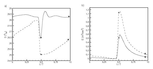
Figure 2. Time series of salinity (a) and kinetic energy (b). -26.9 m, - - 3.84 m; + - 0.5 T, x - 0.95 T.
